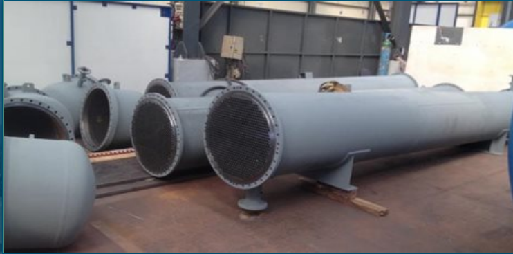
Shell & tube heat exchangers 01/10-TRL-ENTR-401 & 02- SKC-EHTR-101
