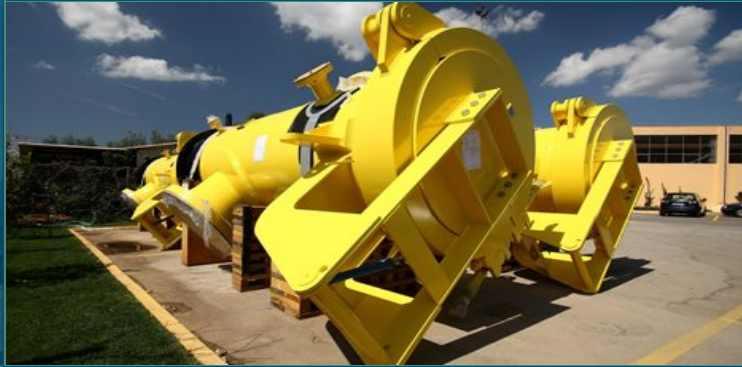
Treated gas filter, solvent gas filters and hot oil filters for Algeria
